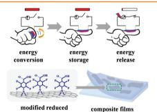
An all-solid-state flexible generator-capacitor film is fabricated by employing the dual role of PVDF-HFP: it serves as both the piezoelectric generator and the polymeric matrix of the capacitor. Chemically modified reduced graphene oxide fillers effectively enhance film permittivity. The film converts low-frequency biomechanical energy to stored electricity and can delayed release the electric signal on demand.
