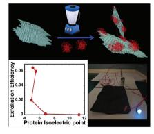
Graphite exfoliates to high-quality, fewlayer graphene when subjected to shear forces in a kitchen blender on a multigram scale, which is assisted by ordinary, edible proteins. Protein charge plays a very important role in the exfoliation mechanism, and the graphene samples are highly conductive. The graphene suspensions in water are stable against temperature (5-50 °C) and a pH range from 3 to 11 for well over a month, and are suitable for biological applications.
