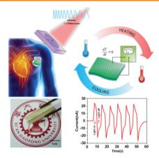
By investigating the pyroelectric performances of poly(vinylidene difluoride) (PVDF) and its remote-manipulability under near-infrared (nIR) irradiation, a flexible battery-less implantable device is proposed. The device is constructed by laminated graphene-PVDF-graphene sandwiches, which can be wirelessly powered and supply regulatable electrical pulses for nerve stimulation by nIR irradiation.
